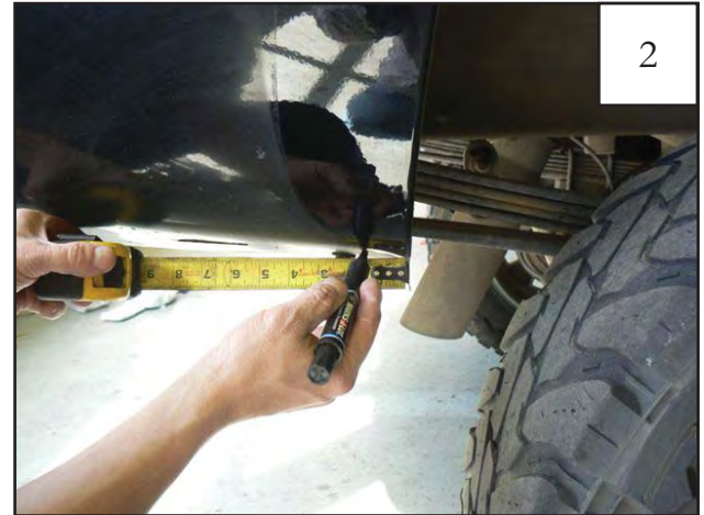
At each end of the wheel well opening, measure in 1.5" and mark.
