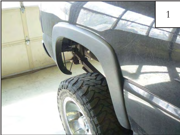
Remove factory flare using a flat blade screwdriver to pry up the head of the fastener.
