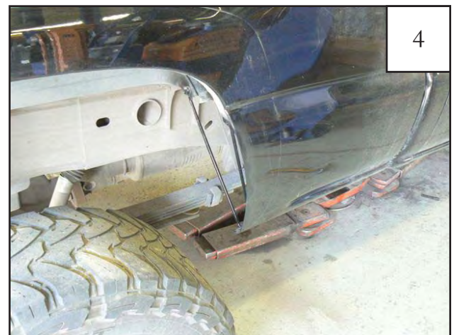
Using a cut off wheel, cut along inside of tapelines. Deburr edges and seal with primer or undercoating.
