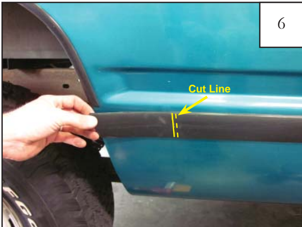
6 Remove the flare and mark a cut line 1/4" beyond overlap line. Use blow dryer or heat gun to heat molding.
