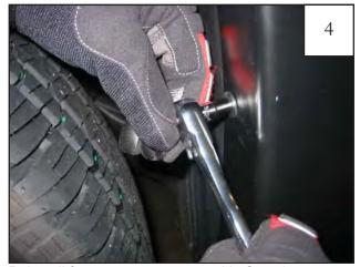
Reinstall factory screws removed in Step 1.
