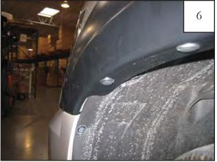
Install a supplied Plastic Push Retainers through forward hole in flare.
