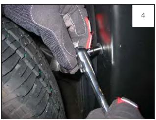
Reinstall factory screws removed in Step 1.
