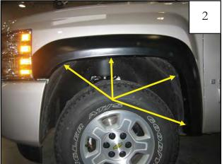
Position flare on fender, and reinstall the four factory screws removed in Step 1. Verify fit and tighten all screws.
