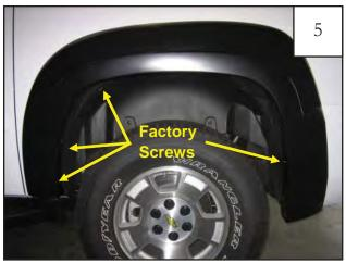
Reinstall four of the five factory screws removed in Step 2.
