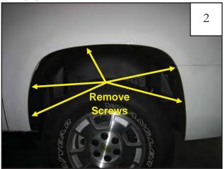
Using a 7mm socket, remove five factory screws. Retain screws for later use.
