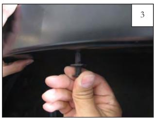
Holding flare in position on fender, install two Plastic Push Retainers in locations shown in Step 4.
