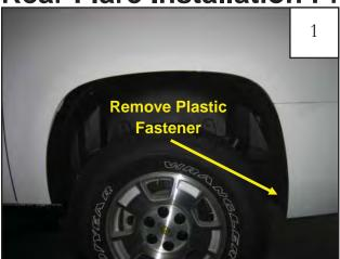
Using a flat head screw driver, remove one factory plastic retainer and discard.
