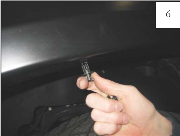
Install two supplied Retainers (RV1-P006).
