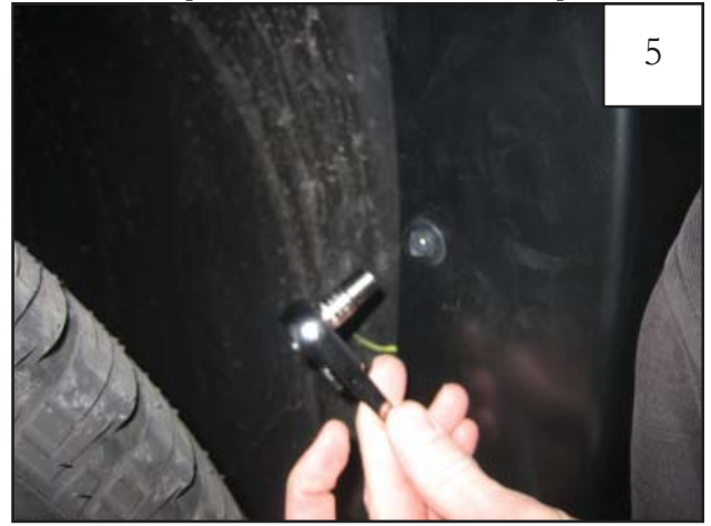
Holding flare in position on fender, reinstall factory screws removed in Step 4. It is helpful to install the one second from bottom first.
