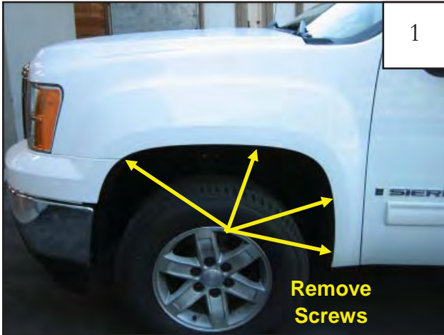
Using a 7mm socket, remove four factory screws. Retain screws for later use.
