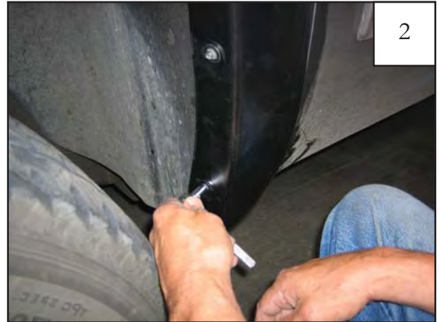
Position flare on fender, and reinstall four factory screws removed in Step 1. If needed, use an awl to locate holes.
