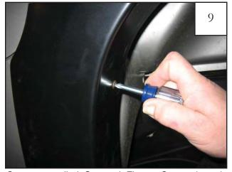
Start a supplied Serrated Flange Screw through each of the remaining holes and into each "S" Clip installed in Step 7. If needed, use awl to locate holes. NOTE: It is helpful to install the two bottom screws first.
