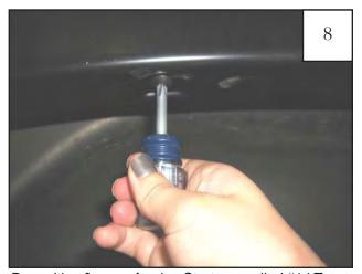
Reposition flare on fender. Start a supplied #14 Truss Head Screw through each topmost hole in the flare, and into each Plastic Clip installed in Step 3.
