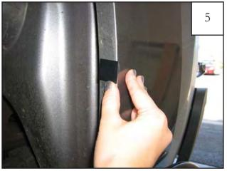
Center a supplied Black Plastic Tab over the six marks made in Step 1, aligning edge of tab with inside of fender lip (tab may extend over outside of fender).
