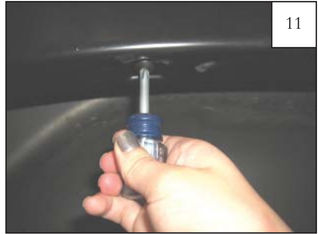
Reposition flare on fender, Start a supplied Screw (SW1-0057) through the two uppermost holes in the flare and into each Clip installed in Step 6.
