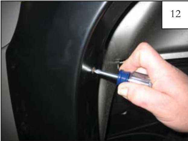
Start a supplied Screw (SW1-0050) through each of the remaining holes and into each Clip installed in Step 10. If needed, use scratch awl to locate holes.
