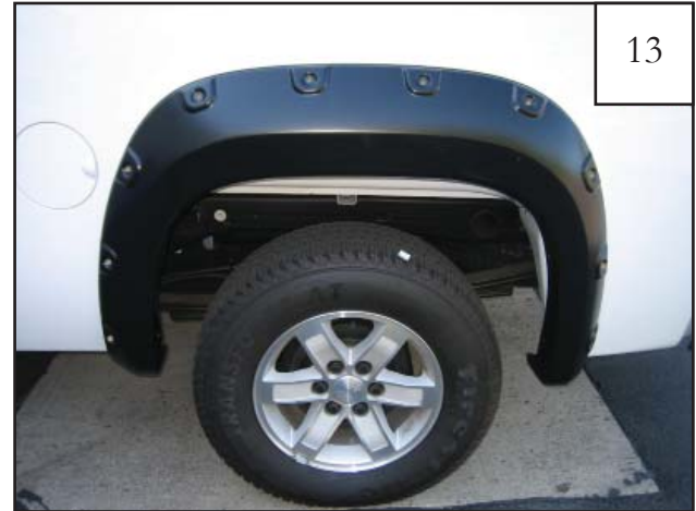
Completed rear flare installation.
