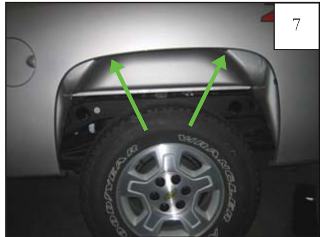
Slide a supplied Clip (CL1-0022) over top two factory holes. Clips may need to be adjusted to align with holes in flare. Note: Some vehicles with inner splash shield will need to remove factory fasteners in indicated locations before installing the clips.
