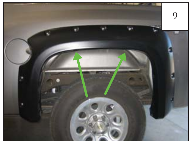
Reposition flare on fender. Start a supplied Screw (SW1-0058) through upper two hole locations and through each Clip (CL1-0022) installed in step 7. If needed, use awl to locate holes.
