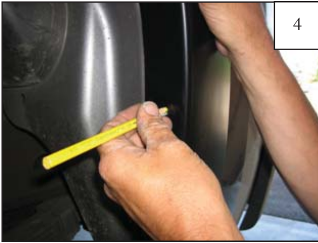
Holding flare in position on fender, use a grease pencil to mark five hole locations.
