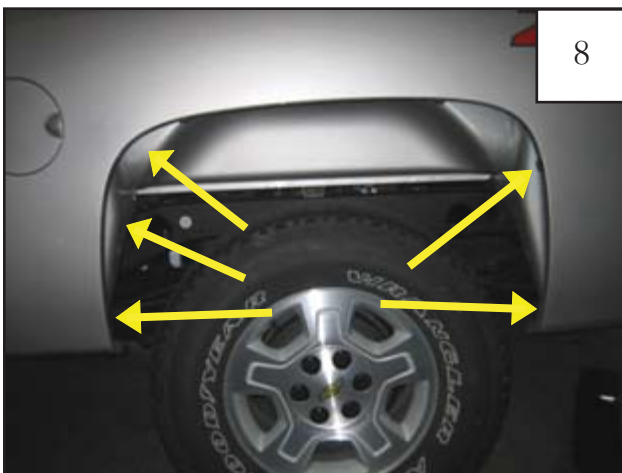
Slide a supplied Clip (CL1-0005) over lower five tabs. Clips may need to be adjusted to align with holes in flare.
