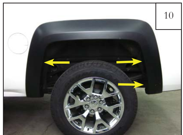
Hole locations to be marked for drilling.
