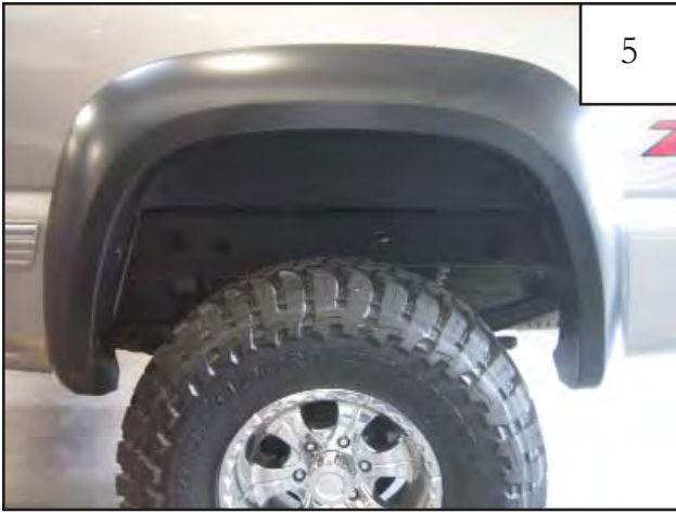
Completed rear flare installation.
