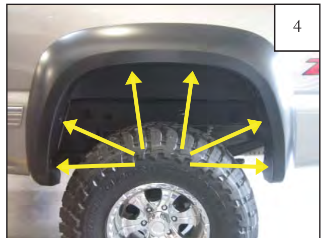
Install six tuflocks using a #2 stubby screwdriver.
