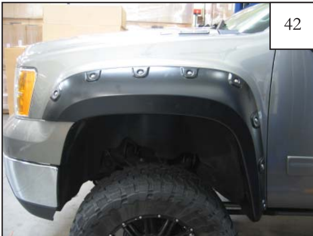
Reinstall wheel. Completed front flare installation.
