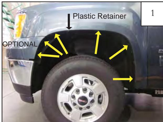
Remove factory mudflap if applicable. Using a 7mm socket, remove four factory screws from wheel well and save for reinstallation. If installing optional bumper piece, remove two front factory screws from bumper and save for reinstallation. *Note: Some models have plastic retainers at top center; remove with pry tool and discard if on vehicle.*
