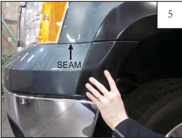
Position flare on fender, aligning bumper piece and flare seams with factory seam. Using a 7mm socket, reinstall factory screws removed in step 1. If needed, use a scratch awl (or similar pointed tool) to locate holes. **DO NOT FULLY TIGHTEN SCREWS**
