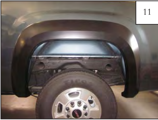
Completed rear flare installation.
