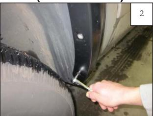
Position flare on fender and start four factory screws removed in Step 1. Verify fit and tighten all screws.
