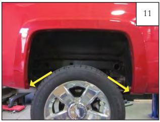
Install supplied screws (SW1-0056) into two lower most holes.
