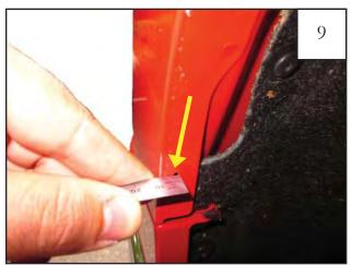
Remove the flare. At the marked locations made in Step 7, measure inward 22mm from the edge of the fender. These are the marks to be drilled.
