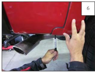
Using a grease pencil, mark the rear bottom fastener using the flare as a guide.
