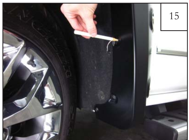
Using a grease pencil or marker, mark one hole location for drilling using the upper rear hole location in the flare as a guide. Note: This step not needed for models with factory installed mudflaps.
