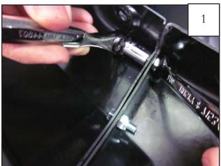
**FOR 1500 MODELS ONLY:** Insert the Screw/Nut assembly (SW1-0005/NU1-0001) through the hole drilled in the end of the Front Main Flare and into the corresponding hole in the Front Bumper Piece. Two places and tighten.
