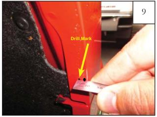
Remove the flare. Using the marks made in step 7 as a guide, measure inward from the outside edge of the fender to verify proper depth of original marked location. Mark must be minium of 10mm in from outside edge of fender, if short, adjust mark to 10mm.
