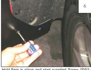
Hold flare in place and start supplied Screw (SW1-0056) through two bottom rear holes in flare and into factory holes in rear of wheel well. *Do not tighten.*
