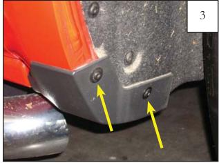
Using a T-15 Torx bit, remove two factory screws in muduguard at rear of front wheel well.
