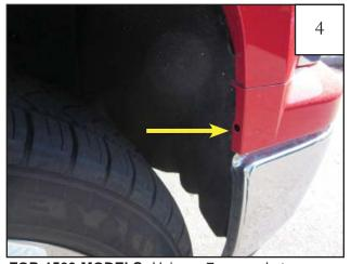
**FOR 1500 MODELS:** Using a 7mm socket, remove factory screw at bottom front of wheel well.
