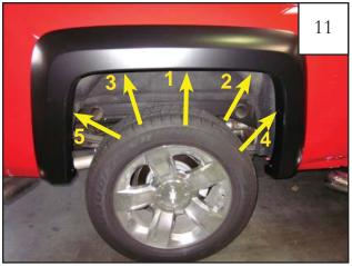
Install supplied self-tapping screws (SW1-0066) into pilot holes in the order indicated. *PRESS FLARE TOWARD VEHICLE AND TIGHTEN ALL SCREWS*
