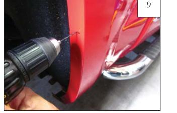
Using a 3/32" drill bit, drill pilot holes at the marks made in Step 8.
