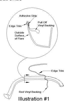
(B) Press edge trim into place along the top edge of the flare in one-foot increments, pulling red vinyl backing free as you continue to work your way around the top edge of the flare.
