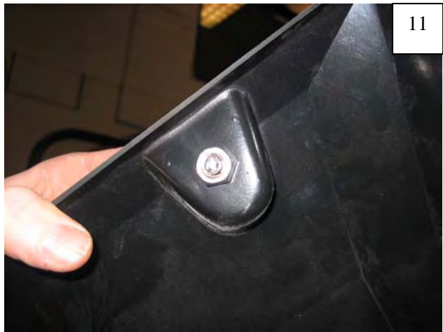
Place a supplied Nyloc Nut on the backside of the screw and tighten using a 1/2" socket and T45 Torx bit. Repeat for all pockets.
