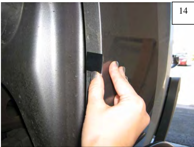
Center a supplied Black Plastic Tab over the marks made in Step 13, aligning edge of tab with inside of fender lip (tab may extend over outside of fender).
