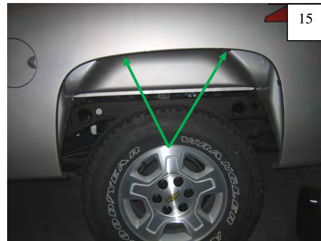
Slide a supplied Speed Clip over top two black tabs. Clips may need to be adjusted to align with holes in flare.
