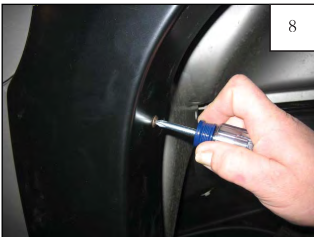
Reposition flare on fender. Start a supplied serrated-flange screw through the hole in the flare, and into each clip.
