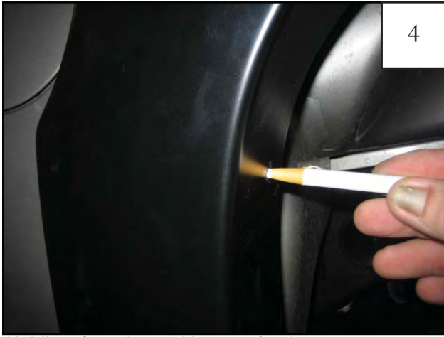
Holding flare in position on fender, use a grease pencil to mark six hole locations.
