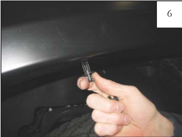
Install two supplied Retainers (RV1-P006).
