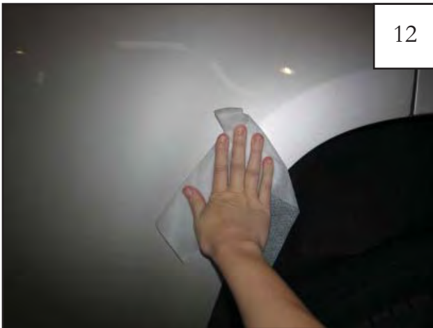
Using a supplied alcohol wipe, clean the area where the door piece will be installed.
