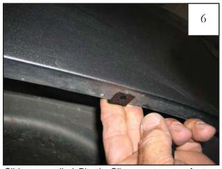
Slide a supplied Plastic Clip over two top factory holes. Clips may need to be adjusted to align with holes in flare. Note: The raised collar on the clip should face upward into the interior of the fender
