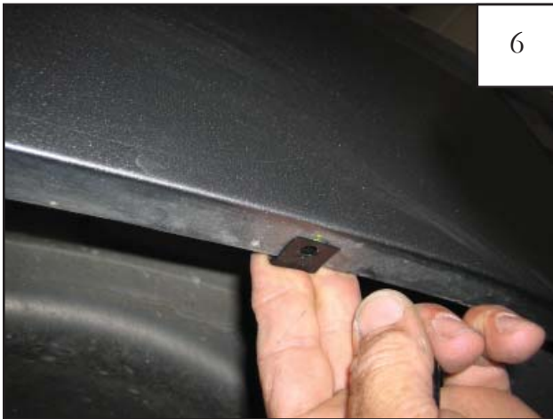
Slide a supplied Plastic Clip over two top marks made in Step 4. Clips may need to be adjusted to align with holes in flare. NOTE: the raised collar on the clip should face upward into the interior of the fender.
