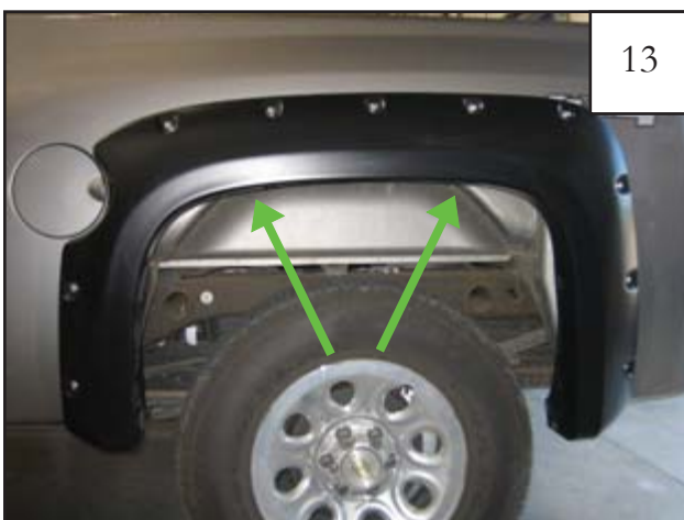
Reposition flare on fender. Start a supplied Screw (SW1-0058) through upper two hole locations and through each Clip (CL1-0022) installed in step 11. If needed, use awl to locate holes.
