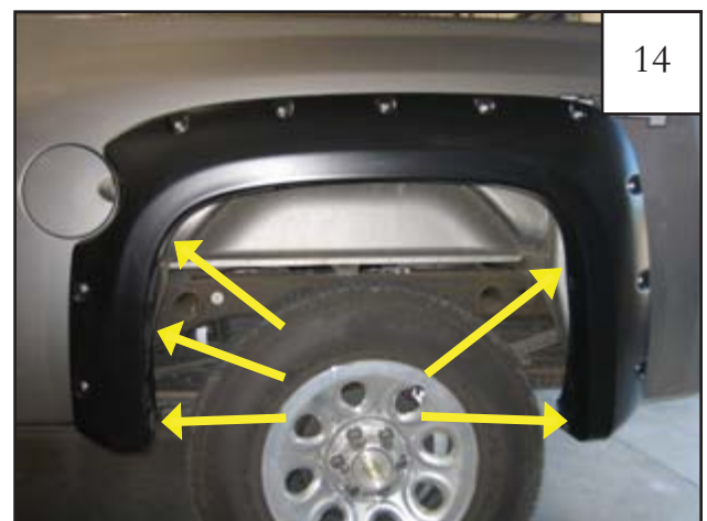
Start a supplied Screw (SW1-0050) through each of the remaining holes and into each Clip (CL1-0005) installed in step 12. If needed, use awl to locate holes.
