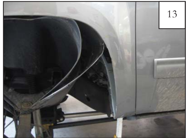
Bend inner fender metal away from fender.
