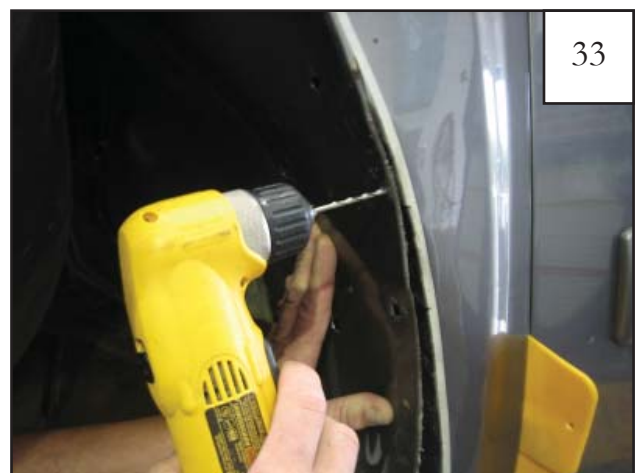
With 3/32" drill bit, drill through mark and the bent tabs of metal behind them for four locations along edge of wheel well.
