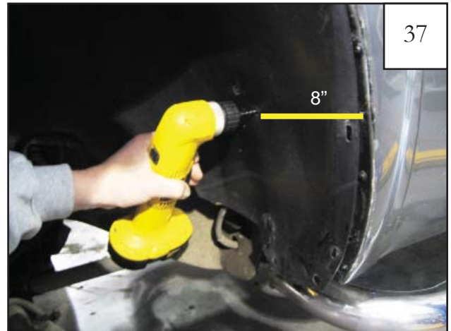
Using a 3/32" bit, drill a hole 8" in from hole in wheel well liner.
