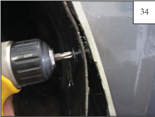
Starting with the top location, fasten inner fender metal to bent tabs of outer fender with Screws (SW1-0056) through holes drilled in last step (4 locations).
