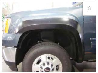
Completed front flare installation without bumper piece.
