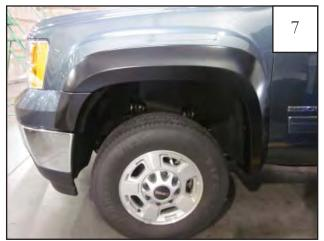
**OPTIONAL BUMPER PIECE:** Completed front flare installation.
