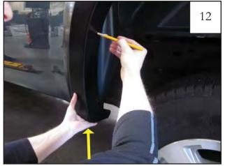
Pushing upward on the flare to ensure proper positioning, use a grease pencil to mark four hole locations. Remove screws installed in Step 11 and remove flare.
