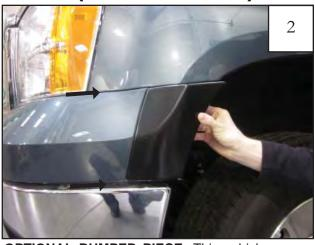
**OPTIONAL BUMPER PIECE:** This vehicle comes with different bumper sizes. If installing the optional bumper piece, verify which piece to use by holding it up to the bumper and making sure it lines up with factory edges and hole locations. After identifying bumper piece, apply edge trim along outer surface.
