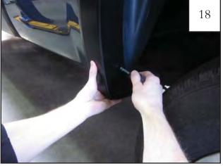
Start a supplied Screw (SW1-0050) through each of the remaining holes and into each Clip installed in Step 16. If needed, use scratch awl (or similar pointed tool) to locate holes. Tighten all screws.
