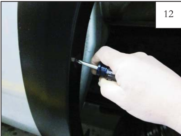
Start a supplied Screw (SW1-0050) through each of the remaining holes and into each Clip installed in Step 9. If needed, use scratch awl to locate holes.
