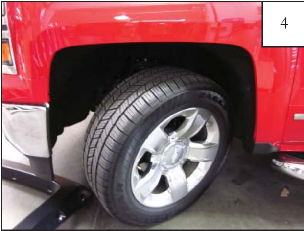
Turn front tire outward for easier installation.
