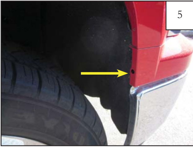
FOR 1500 MODELS: Using a 7mm socket, remove factory screw at bottom front of wheel well.
