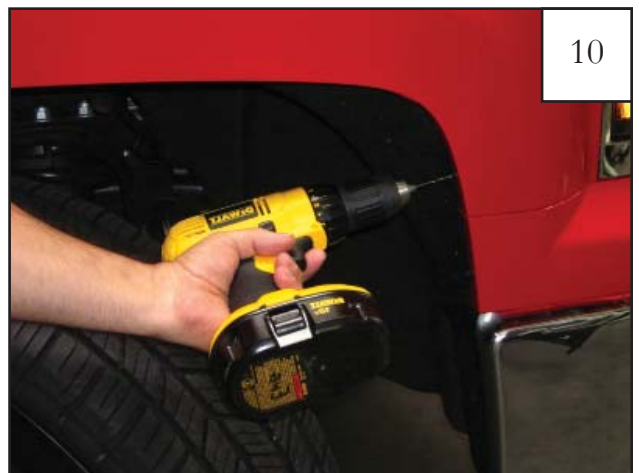
Using a 3/32" drill bit, drill pilot holes at the marks made in Step 9.
