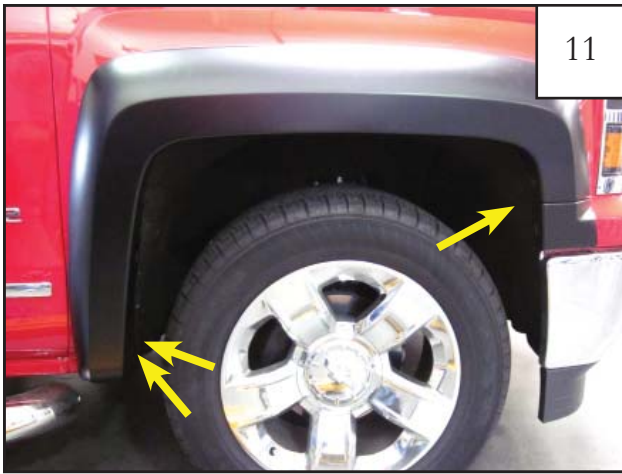
11 Locate flare into position on vehicle. Install supplied screw (SW1-0056) through two bottom rear holes in flare and into factory hole in front of wheel well.
