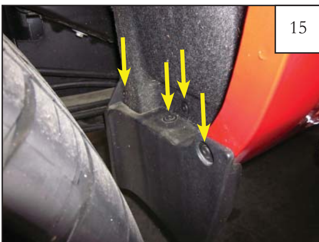
15 Using a T-15 Torx bit socket wrench, remove the four factory screws from the factory forward splash guard. Remove splash guard and discard.
