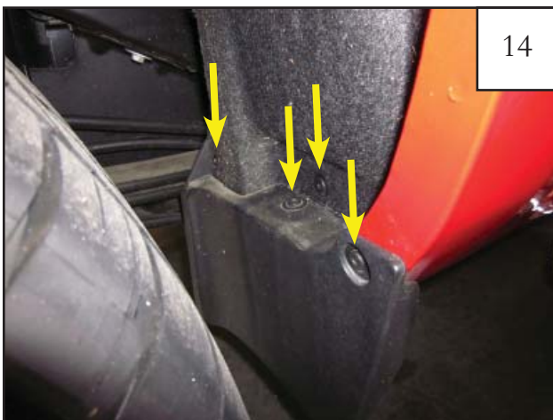
Using a T-15 Torx bit socket wrench, remove the four factory screws from the factory forward splash guard. Remove splash guard and discard.
