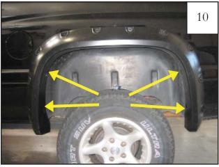
Using a right-angle drill with a #2 Phillips bit, drill four supplied Screws (SW1-0066) through plastic of fender flare and into sheet metal of fender using the indents in the flare as a guide.
