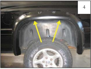
Position flare on fender, pushing flare tightly against fender. Using a right-angle drill with a #2 Phillips bit, drill two supplied Screw (SW1-0066) through plastic of fender flare and into sheet metal of fender using the indents in the flare as a guide.
