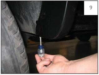
Using a Phillips screwdriver, start two supplied Screws (SW1-0049) into Clips installed in Step 8. If necessary use an awl to locate holes and adjust clips. *Note: Do not tighten. Check flare position and make sure flare fits into style line.*
