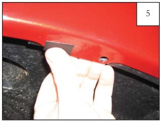
Install two tabs (MT1-0002) over factory holes. There are two factory holes near the rearward arrow. The correct hole for install is the one more toward the front of the vehicle.
