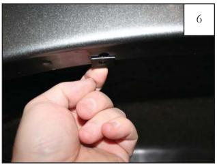
Install #10 U-Clip over existing factory holes. There are two holes at the top center location. The hole for proper installation is the one toward the front of the vehicle. NOTE: The clip may fit over the lip loosely. This can be fixed by pinching the clip more tightly to the vehicle.
