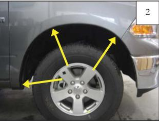
Remove three factory installed screws with 8mm socket wrench.
