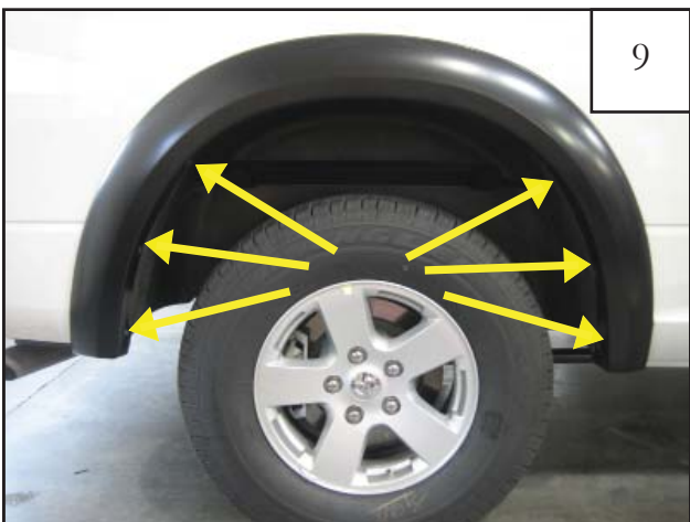
Hold flare in place while you start six additional supplied screws using a Phillips Head Screwdriver. Do not tighten.
