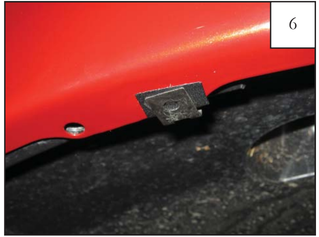
Install U-Clip over plastic tab.
