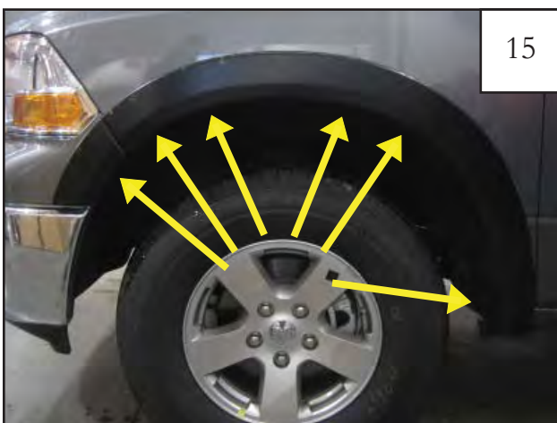
METAL BUMPER ONLY: Press firmly on flare and tighten all screws.
