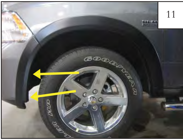
PLASTIC BUMPER ONLY: Additional kit supplied screw locations. See step 12 & 13.
