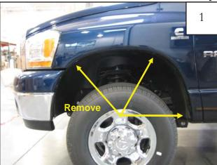
Using an 8mm socket, remove three factory screws from wheel well. Retain for future use.
