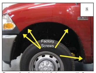
Remove four factory installed screws with 8 mm socket wrench.
