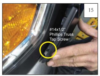
When fitting flare on vehicle, first position front piece. The #14x1/2" Phillips Truss Tap Screw hooks behind where folded 1"x1.5" Black Tab was installed in step 6.
