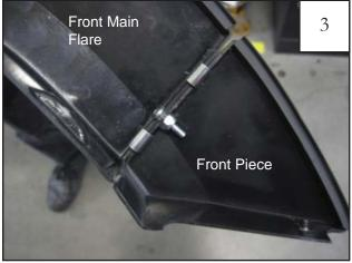
Secure pieces with two SS U-Clips to prevent rotation out of alignment after installation.
