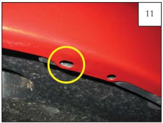
At location indicated in step 10, there is a lip with two factory holes. One hole is a circle and one is an oval. The 1"x1.5" Black Tab and #10 U-Clip will be installed over the oval. The oval is the hole more toward the front of the vehicle.
