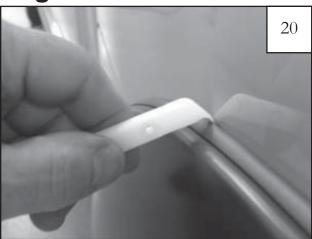
Using supplied Edge Trim Tool, seat Wiper Style Edge Trim against vehicle by hooking curved end under edge trim at one end of flare. Next, slide around outer edge of flare to the other end.
