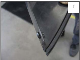
Using dimple in front piece as a guide, drill a 1/8" hole and install a #14x1/2" Phillips Truss Tap Screw through the drilled hole.
