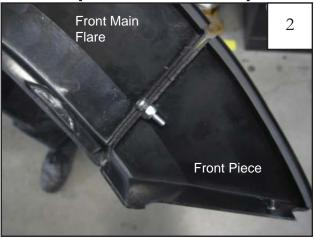
Bolt front main flare and front pieces together with #10-24x3/4" Phillips Pan Machine Screw and #10-24x3/8" Nylock Nut. Use a 3/8" wrench to hold #10-24x3/8" Nylock Nut in place.
