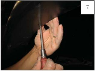
Using a #2 Phillips Screwdriver, insert a supplied Truss-Head Screw through existing holes in flare and into holes in clips (4 places).
