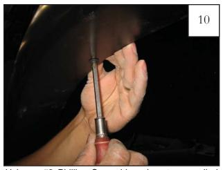
Using a #2 Phillips Screwdriver, insert a supplied Truss-Head Screw through existing holes in flare and into holes in clips (4 places).
