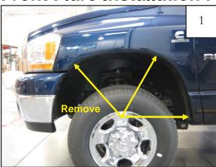
Using an 8mm socket, remove three factory screws from wheel well. Retain for future use.
