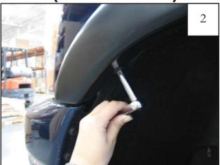
Holding flare in position on fender, reinstall screws removed in Step 1.
