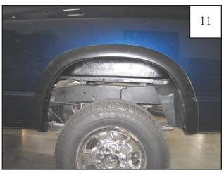
Make sure flare is positioned correctly on vehicle. Tighten all screws.
