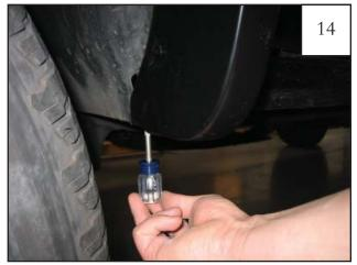
Using a Phillips screwdriver, start two supplied Screws (SW1-0049) into Clips installed in Step 13. If necessary use an awl to locate holes and adjust clips. *Do not tighten. Check flare position and make sure flare fits into style line.*
