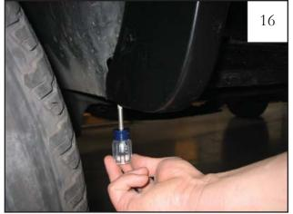
Using a Phillips screwdriver, tighten screws started in Step 14. If necessary use an awl to locate holes and adjust clips.
