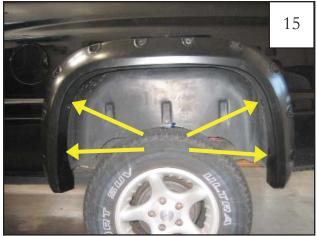
Using a right-angle drill with a #2 Phillips bit, drill four supplied Screws (SW1-0066) through plastic of fender flare and into sheet metal of fender using the indents in the flare as a guide.
