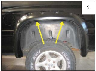
Position flare on fender, pushing flare tightly against fender. Using a right-angle drill with a #2 Phillips bit, drill two supplied Screw (SW1-0066) through plastic of fender flare and into sheet metal of fender using the indents in the flare as a guide.
