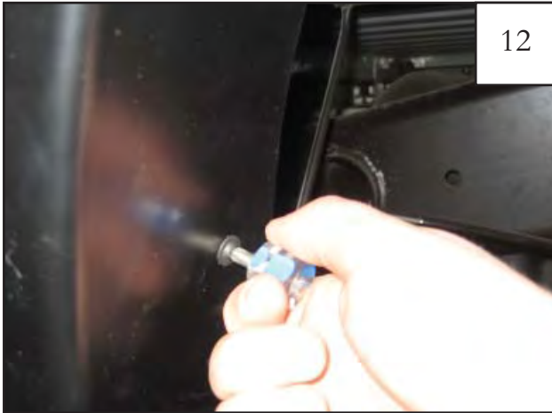
Using #2 Phillips Screwdriver, insert a supplied Screw (SW1-0056) through existing holes in flare and into holes in clips (4 places).
