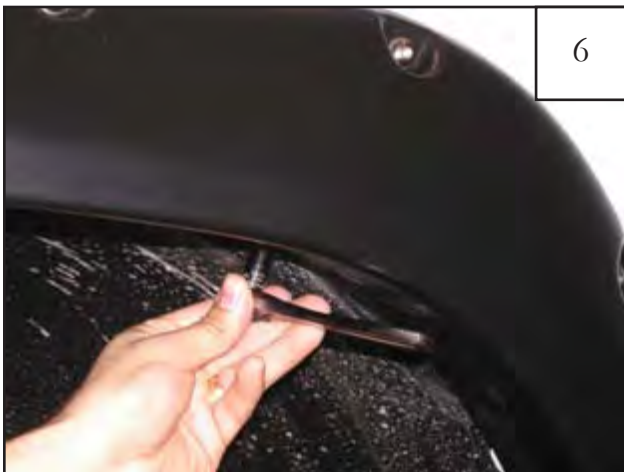
Holding flare in position on fender, reinstall screws removed in Step 5.
