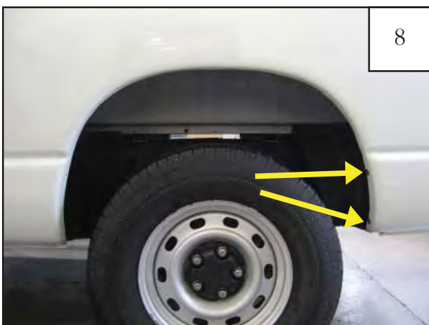
Using an 8mm socket, remove two factory screws from rear of wheel well. Save for reinstallation.
