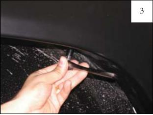
Holding flare in position on fendar, reinstall screws removed in Step 2.
