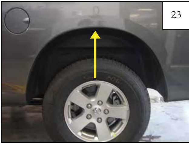
Install speed clip in this location. See steps 24-26.
