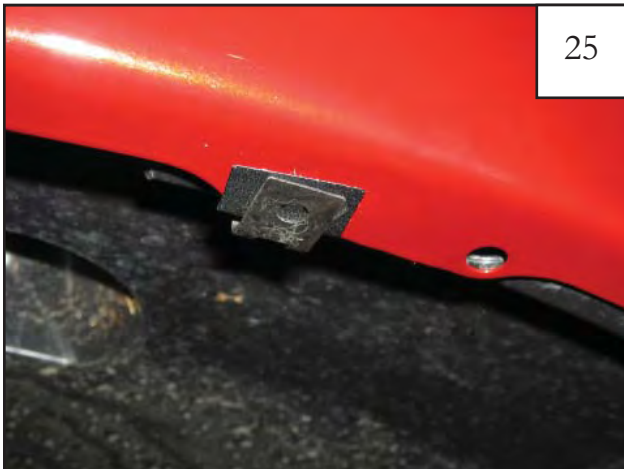
Install speed clip over plastic tab.
