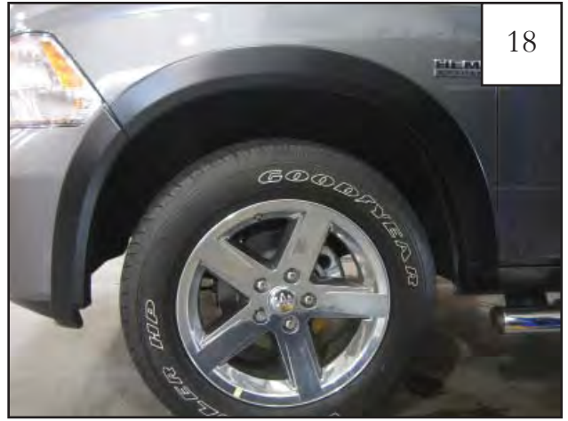
PLASTIC BUMPER ONLY: Completed front flare installation.
