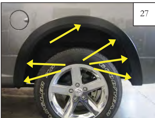
Supplied screw (SW1-0056) locations. See steps 28 & 29
