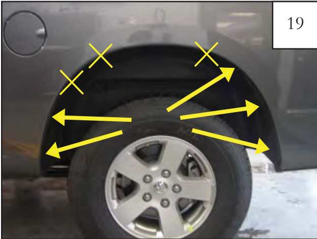
Remove these five factory installed screws using an 8mm socket wrench. X's indicate a factory screw that will not be removed.
