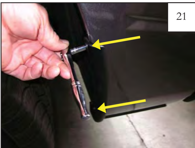
Using a socket and wrench remove the two factory screws from the plastic wheel well piece.
