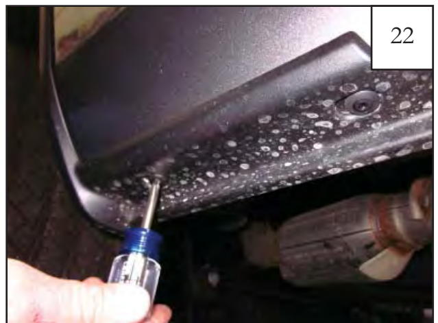
Using a screwdriver remove the two factory fasteners from the bottom side of the plastic wheel well piece. Remove plastic wheel well piece at this time.
