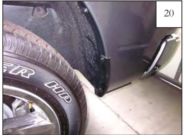
2013 Models and up : You will need to remove the plastic factory wheel well piece from the rear of the wheel well. Please follow steps 21 & 22.
