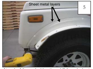
At each of the marked locations drill through sheet metal using a 3/16" bit. If necessary, drill through both layers of sheet metal because they overlap.
