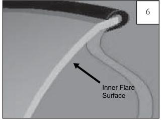
Peel 2-3 inches of red vinyl backing away from Edge Trim (GP1-0008) tape. Applying adhesive side to inner side of flare, affix edge trim to top of flare (portion that comes in contact with vehicle). Press edge trim into place along edge in 1-foot increments pulling backing as you go.
