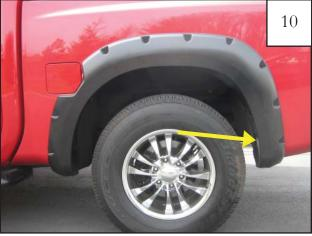
Hold flare in position on fender with moderate pressure. Line up the lowest hole in fender with the hole in flare and start the factory screw. *Do not fully tighten screws*.
