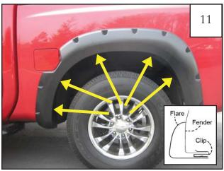
Install five Clips (CL1-0005) over fender lip, lining up the hole in Clips with the holes in flare. Start Screws (SW1-0050) in each Clip. *Do not fully tighten screws*.
