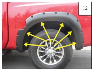
Insuring the flare is properly located on fender, apply moderate pressure to outside surface of flare, tighten all screws, beginning with the factory screw working toward the front of the fender flare.
